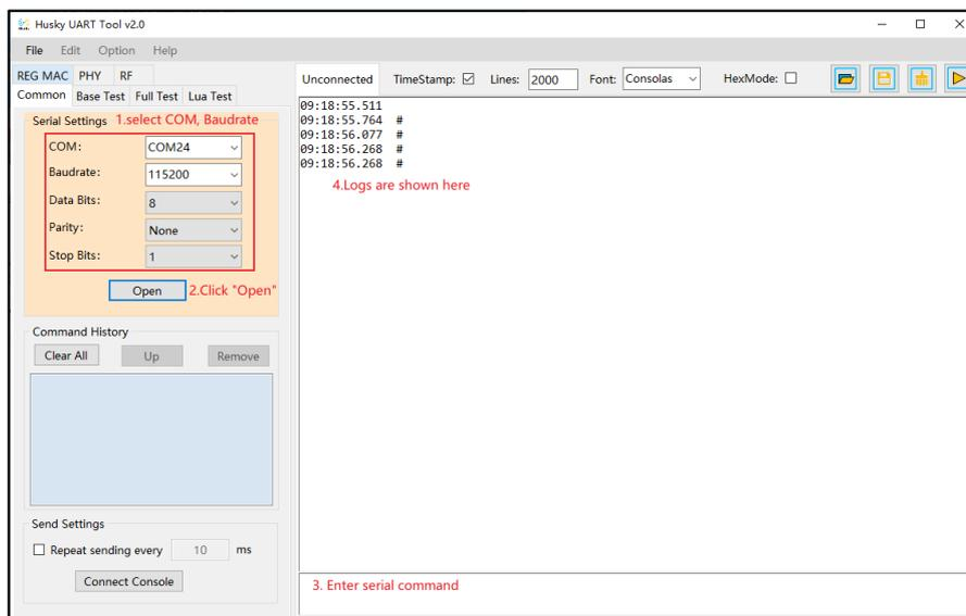
2. Click the button to connect the serial port. Press "**Reset**" at the side of the development board, and the serial port output box displays the log information, as shown in [Figure 4-2. Serial port boot information](#). At this moment, left-click in the serial port input box and press "**Enter**" on the keyboard, and the log displays "**#**":
